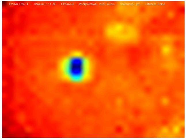
This image is of a coin buried 2cm under sand in the evening, clearly showing the camera's detection capabilities and proving that the concept of detecting the mines works. The colour-grading we are using here is where the blue part shows a higher temperature area, different from the first picture. We can see that the plate is hotter than the soil. The distance between the camera and the soil surface is around 30cm.
