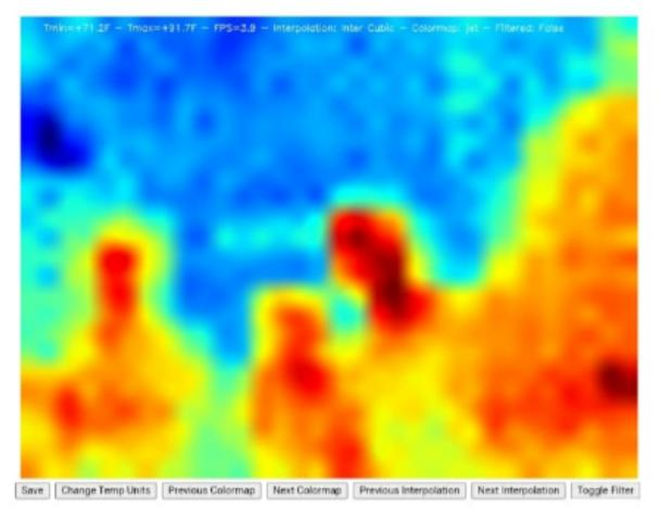
This is the test image where we can see three subjects in the frame and the thermal camera detecting their heat signature. In this picture, the colour grading we used is such that the higher temperature area is red.
